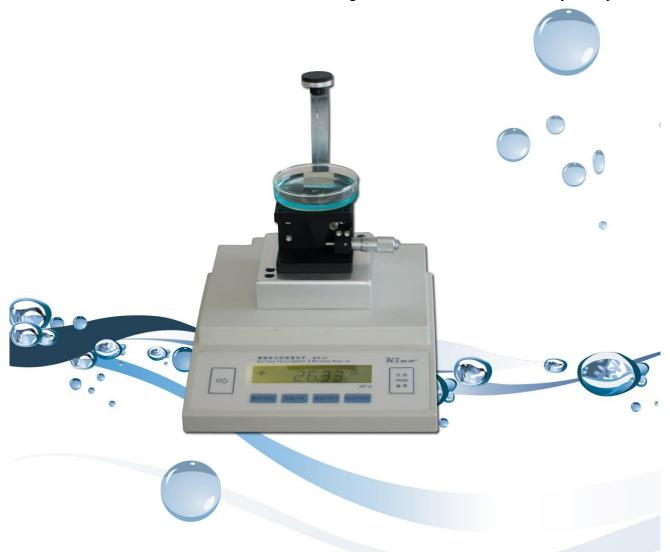
Surface tensiometer model A3 is manual standard version standalone instrument that equipped with analytical balance and high precise positioning stage. It can be used to measure surface tension of liquids based on Wilhelmy plate and Du Noüy ring methods rapidly and simply.
